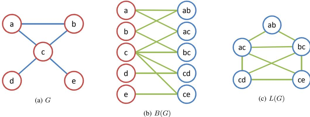
Figure 1: An example graph  $G$  and its corresponding bipartite feature graph  $B(G)$  and line graph  $L(G)$ . In (b) and (c), the blue nodes represent the edges in  $G$ ; e.g., edge  $ab$  represents the edge connecting  $a$  and  $b$  in (a).
